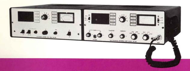
The TM-350 Transceiver is an efficient combination of the TM-125 Transceiver driving the TMA-350 Linear Amplifier. Both units are housed in identical cabinets suitable for desk top or vehicle mounting and operate in the 1.6 to 26 MHz frequency range off a 115 VAC power source. Eight simplex, or on special order, eight half-duplex channels can be provided with better than one ppm/OC stability for each channel.
