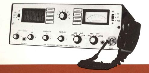
The TM-125 Transceiver is a completely self-contained unit measuring 5½ X 14½ X 16 inches and capable of up to eight channels transmit, receive or transceive. In addition, on special order a 16—channel oscillator board can be provided, making possible half-duplex operation (transmit on one frequency and receive on another).
