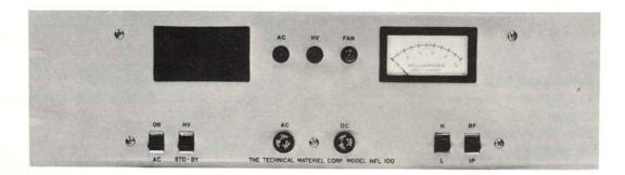
The Model HFL-100 is a high quality linear amplifier, designed to operate in the 1.6 to 26 MHz range, and broadbanded (no tuning controls) in two ranges. It provides approximately 50 watts average and 100 watts PEP output when driven by any exciter capable of 50 to 100 milliwatts RF drive. Although the nominal range is 1.6 to 26 MHz, the amplifier is useable from 400 KHz to 30 MHz at reduced efficiency. On special order, it can provide 200 watts PEP output when optimized over a narrower range.
