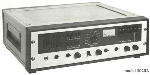
The Marine receiver Model 3020A is a rugged, state-of-the art, highly stable, maritime and general purpose radio receiver. It is a completely solid state, dual conversion, superhytrodyne design providing continuous frequency coverage from 15kHz to 29.9999 MHz. Frequency selection is accomplished by a digitally controlled synthesizer.
