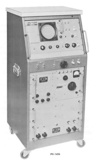
TMC Model PTE-3 (AN/GRM-33A) Spectrum Analyzer is a versatile test instrument designed for RF spectrum analysis. Visual display of RF signals in tuning and aligning single sideband exciters and transmitters provides analysis of intermodulation distortion, hum and noise. Manual Sweep Control provides detailed analysis of any portion of the RF spectrum within the frequency range of 2 to 64 Mcs.
