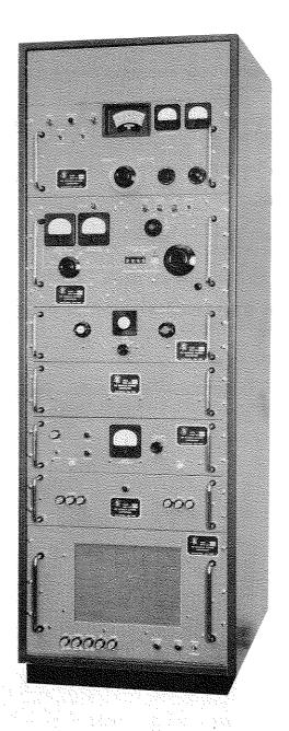
The TMC Model CPO-1, Controlled Precision Oscillator, is a stabilized general purpose frequency generating system adjustable to 320,000 frequencies over the frequency range of 1.75 to 33.75 megacycles in 100 cycle steps with a basic stability of 1 part in 108 per day.
