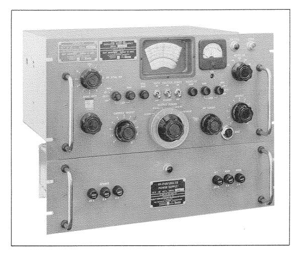
The TMC Model SBE-3, Mode Selector, Transmitting, is a universal exciter permitting the transmission of any intelligence on Single or Double Sideband, with or without carrier.
