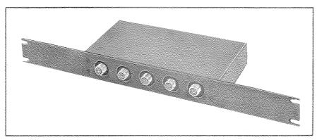
The TMC Models HFD and LFD are passive antenna distribution units consisting of a specially designed broadband transformer with a single input and four outputs. These units allow four receivers to operate from a single antenna with minimum interaction and insertion loss.
