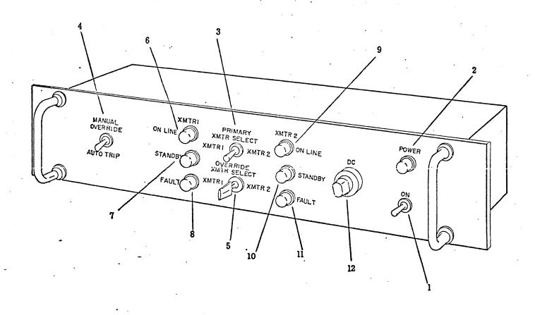
Figure 2-1. Location of Operating Controls and Indicators
