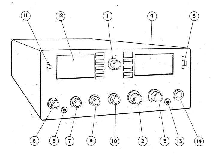
Figure 2-1. Front Panel Controls and Indicators
