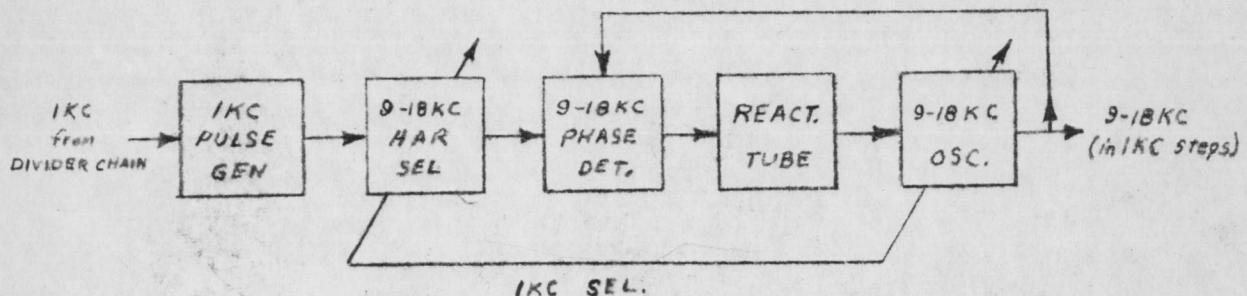
An oscillator is locked on a harmonic of a 1 kc pulse. The 1 kc from the divider chain triggers a pulse generator. This pulse is rich in harmonics from 9 to 18 kc. The desired harmonic is selected and compared with the output frequency of the 9-18 kc oscillator in a phase detector. The dc output voltage of the phase detector synchronizes the oscillator to the selected harmonic.
