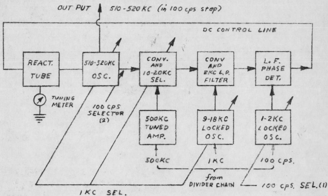
The output frequency is controlled by the kc selector and two 100-cycle selector switches. The kc selector steps the frequency of the 510 to 520 kc oscillator, the 10 to 20 kc selector, and the 9 to 18 kc locked oscillator in 1 kc increments. The 100-cycle selector (1) determines the frequency of the 1 to 2 kc locked oscillator in 100-cycle steps and the 100-cycle selector(2) varies the 510 to 520 kc oscillator frequency between the kc settings.
