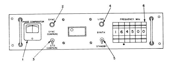
Figure 2-1. Receiver Stabilization Unit, Model RSU-1, Controls and Indicators
