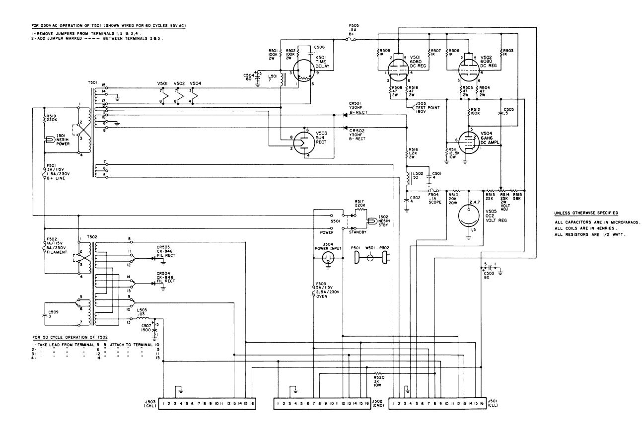
Figure III(F)-8-1. Power Supply CPP-2, Schematic Diagram
