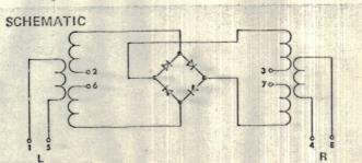
The I-port is formed by externally connecting pins 2 and 6 together and pins 3 and 7 together. Best performance is obtained by grounding the 2, 6 side.
