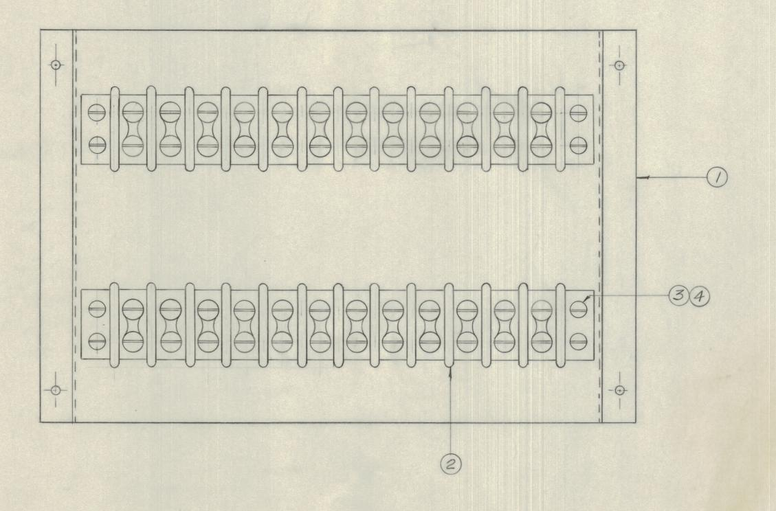
8 4 NTH0632BC8 NUT 8 3 SCBS OG 32BNIO SCREW 22 TERMINAL STRIP 1 1 MS-10158 TERMINAL MOUNTING BRACKET REQ. ITEM PART NO. DESCRIPTION TMC(Canada)LIMITED STOCK SIZE TERMINAL BOARD ASSBLY MATERIAL WEIGHT PER PC. L. MARION TYPE & TEMPER DRAWN ELEC. DES. APP. MECH. DES. APP. HEAT TREAT, SPEC. CHECKED FINAL APPROVAL A-10086 FINISH & SPEC. NO.
